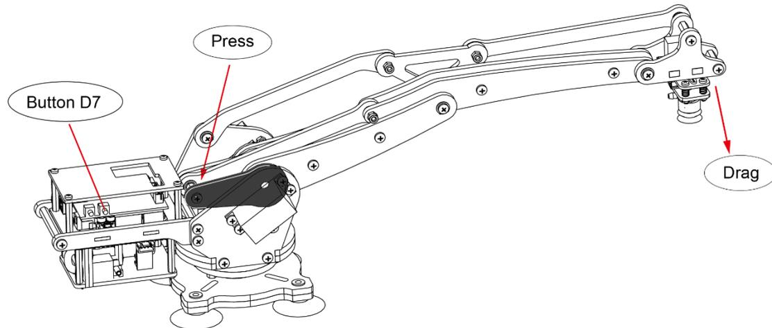
Press **Button D7** once and move your hand out of the way. The uArm will finish its Calibration and go back to its zero position.
