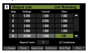
By editing the single-step setting value and duration, the list function can generate multiple sequences to meet complex test requirements. The user can edit the sequence by 50 steps natively or import the list sequence file via USB for multi-step running. Through panel operation, 8 sets of built-in list sequence output control can be achieved, providing users with simple power programming capabilities.
