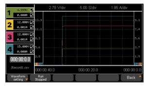
The SPD4000X series programmable linear DC power supply is equipped with a 4.3-inch, true color TFT-LCD display screen with a resolution of 480×272. 4 channels of voltage and current waveform run chart can be set, allowing users to dynamically observe changes in the output state more intuitively.
