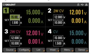
The highest resolution of 1mV/1mA (SPD4000X), provides excellent setting and read back accuracy. This ensures accurate output even with minimal voltage or current changes. This is impossible for a low-resolution power supply.
