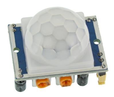
HC-SR501 is based on infrared technology, automatic control module, using Germany imported LHI778 probe design, high sensitivity, high reliability, ultra-low-voltage operating mode, widely used in various auto-sensing electrical equipment, especially for battery-powered automatic controlled products.
