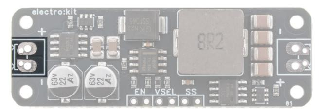
The module can be supplied with a DC voltage between 4 and 40V, but must be 1V higher than the selected output. For 3.3V output, VIN must be  $\sim$ 4.5V and for 5V out,  $\sim$ 6V.
