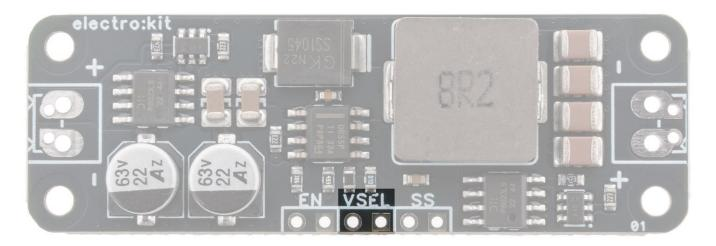
These two pins are used to select one of two pre-programmed output voltages. If left unconnected, the module will output a nice 3.3V. If shorted, it will output 5V. Simple!
