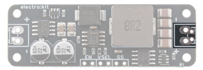
The output pins are identical in size as the input and will work with the same connectors. The output has the same type of protection as the input and will protect the module from backfeed, which means that it can be used in applications where more than one source is used (e.g. when a device can be powered from either a DC-jack, a USB port or both at the same time).
