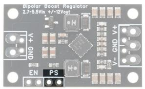
Bridge the two "EN" pins to disable the regulator and reduce the quincent current to 1uA.
