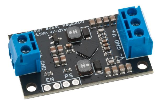
Power supply module based around a dual output switching voltage regulator, to provide a bipolar output voltage of -12V and +12V. Very useful for powering OP-amplfifiers, ADCs, DACs, and other analog circuits that require both positive and negative voltages.
