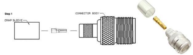
Each connector consists of one body assembly (jack), one rear ferrule (crimp sleeve), and one center pin (jack contact).
