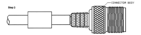
Slide the ferrule (placed on the coax at the beginning of Step 2) over the braid and completely up against the connector body. Using the 0.429 hex of the 7505-DIE-400 installed into the 7505-HANDLE ratcheting crimp handle, crimp the ferrule at the location shown in the picture below (on the ferrule, but right up against the main body of the connector).
