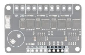
The logic supply voltage and control inputs are all arranged on one side of the board. The connector pitch is 2.54mm and will fit any standard pin header.
