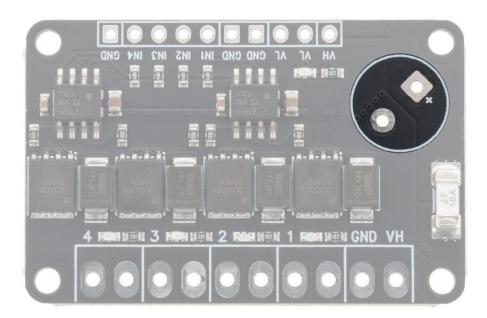
The board has space for a large electrolytic capacitor that can be installed if necessary. The capacitor is normally not required for small loads and is not included. The pattern will fit capacitors with 5mm pitch and a diameter of 10mm (max 12.7mm). Be observant of the capacitor voltage rating! The working voltage should be higher than FET voltage supply with some margin and the capacitor should be a low impedance model.
