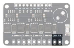
The connections for channels 1 to 4 and FET voltage supply are made using 3.5mm pitch screw terminals (or by soldering wires directly to the board).
