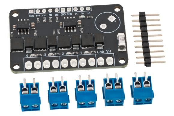
EKM013 and EKM014 are two small modules with two (EKM013) and four (EKM014) powerful FETs for driving heavy loads. The FETs are controlled by a very fast driver IC from Ti that can toggle the transistors fully on and off at extremely high frequencies.
