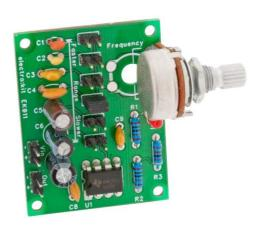
\* Supply voltage: 3 - 15VDC \* Max output current: ±200mA
