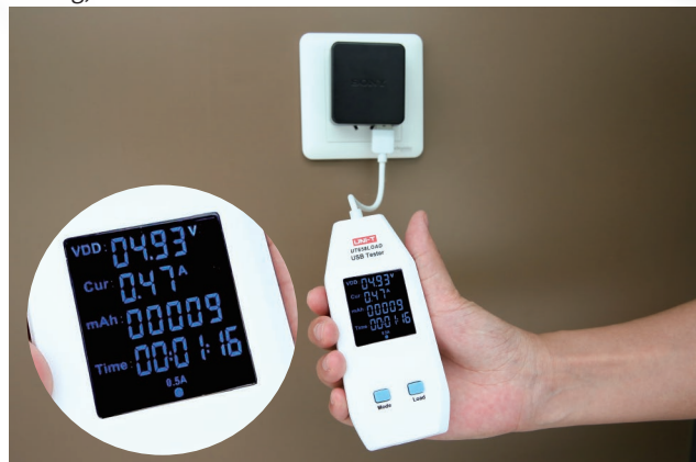
Tester with electronic load (UT658 LOAD)
