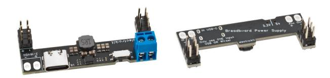
Take note of the "+" and "-" markings when plugging the module into the breadboard. They should align with the red and blue lines on the power rails on the breadboard to avoid confusion.
